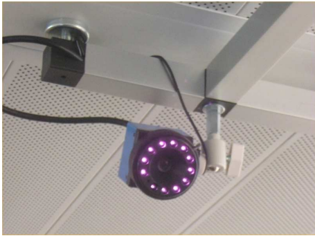
Figure 1: Firewire IEEE 1394 camera with additional IR diodes.
