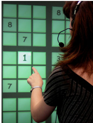
Fig. 4. Solving a Sudoku puzzle using multimodal interaction like the fusion of pointing and speech recognition within the rendering application.
